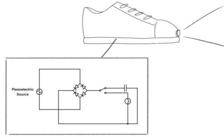
If the LED is switched on, the energy stored in the NiMH battery can flow to the LED and light up the LED bulb. If there is not enough energy, the energy generated when the piezo crystals are pressed can also be used to light up the bulb.
