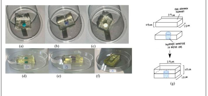
Aerial and side views of the double-layered egg albumen hydrogel bandage with its center cross-linked with (a)(d) copper-calcium (b)(e) copper-zinc (c)(f) calcium metal ions (g) Illustrations of the design of a double-layered hydrogel.
