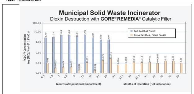
After full installation of those catalytic filters bags, there is only clean gas left. From this bar chart, we can prove that the catalytic filters work.
