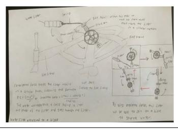
Before making this prototype, we have made 2 previous prototypes which had containers that were permanently sealed, meaning that materials kept inside the filter cannot be replaced. In this prototype, we added an option to change fresh materials by using screw top capsules thus more practical.
