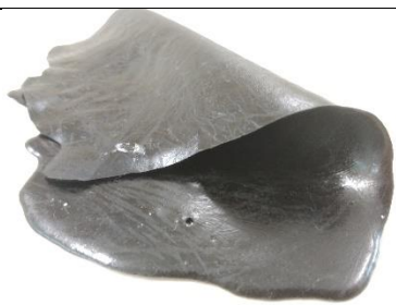
Final product made from waste cooking oil, citric acid and coffee ground
