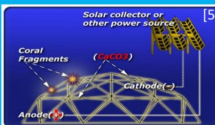
Substratum enhancement with electricity encourages the precipitation of calcium and magnesium on artificial substrata[6], which increase the calcification of coral polyps, boosting colony growth and resilience to stressors.[3]
